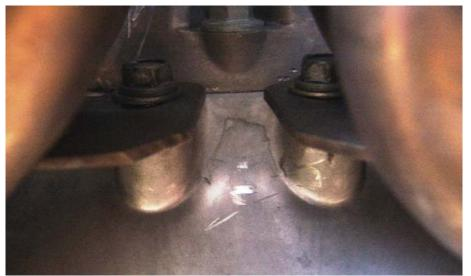
Figure 3: Vertical bell housing mounting bolts (factory manifold studs can also be used)
