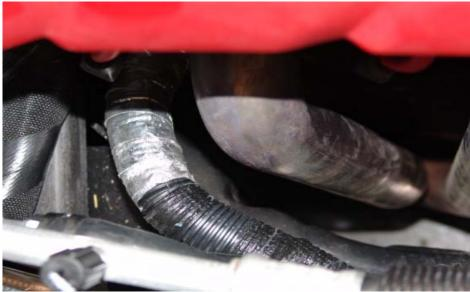
Figure 2: Passenger side wiring harness after being relocated
