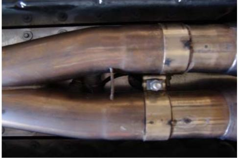
Figure 4: X-pipe location with hole drilled for 02 sensor wires (front is to the right).
