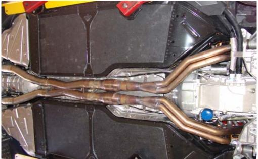
Figure 5: Fully installed LG Long Tube header system on 2006 Z06.
